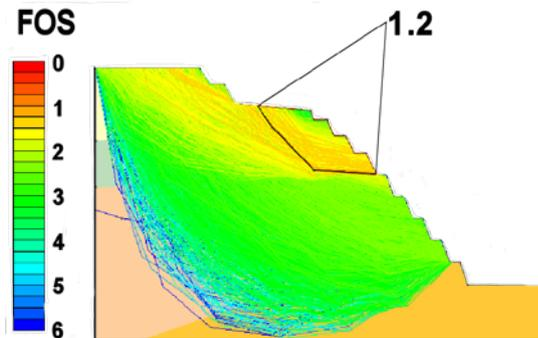
Fig. 3 FOS using limiting equilibrium analysis. (the critical surface shown has FOS = 1.21).
