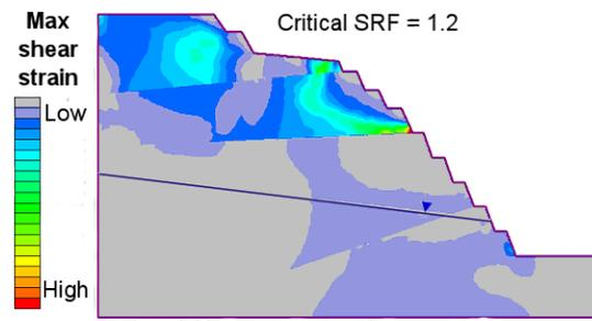
Fig. 4 Modelled strength reduction factor for the mid-west slope.
