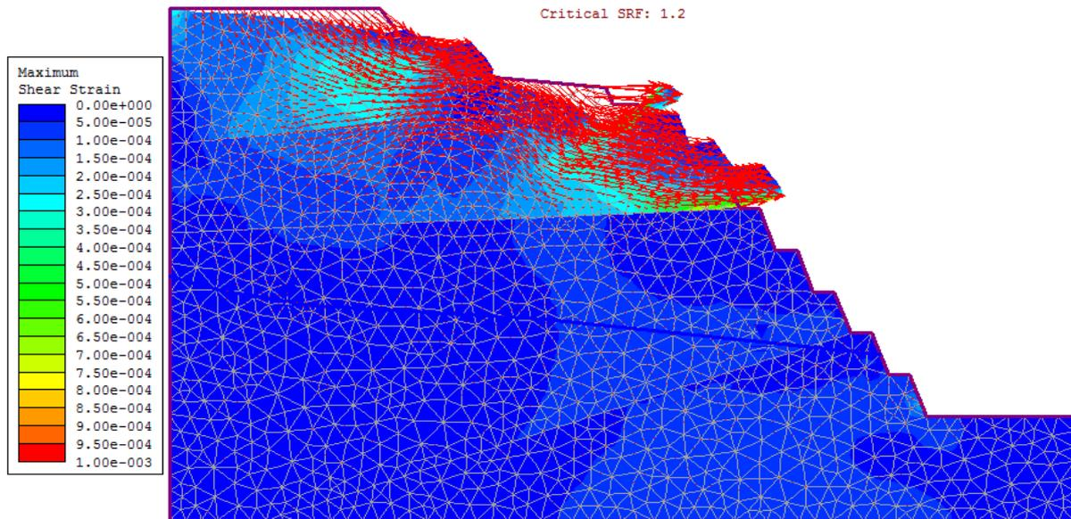
Fig. 5 Modelled displacement vectors of deformation showing the possible directions of block rotation and sliding modes.
