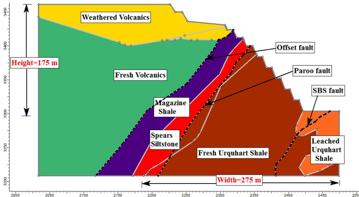
Fig. 2 Slide model of the Handlebar Hill west slope
