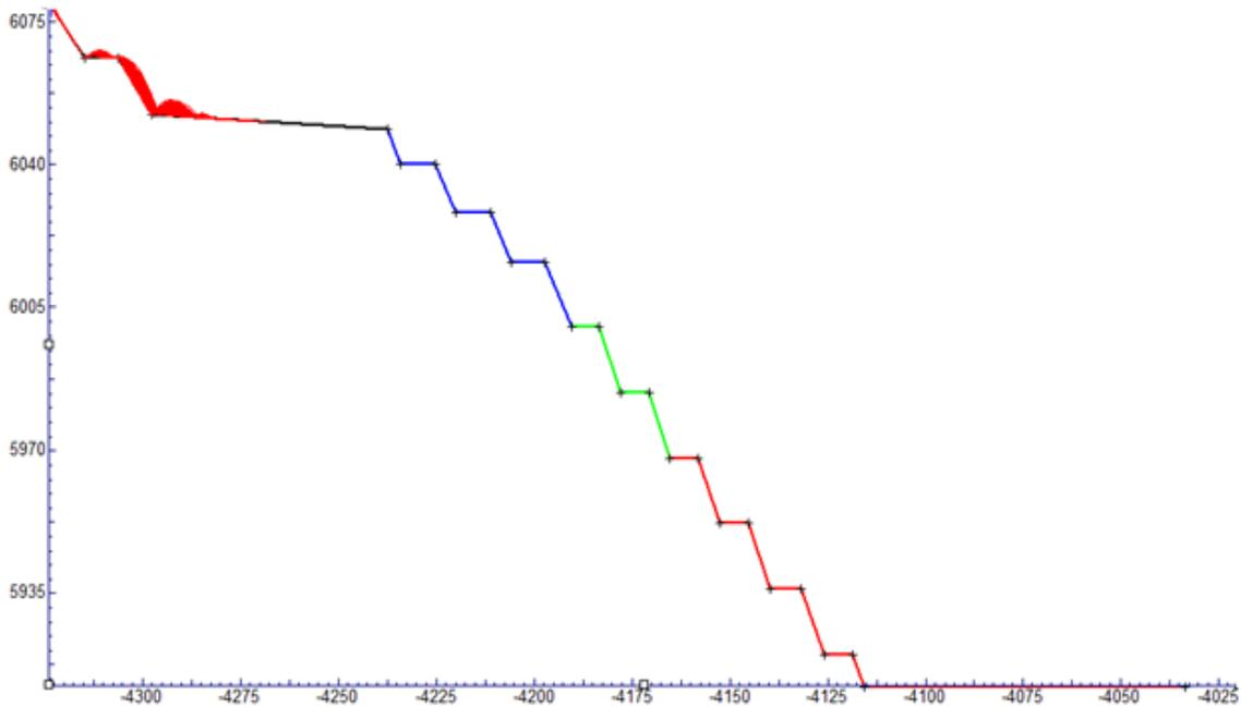
Fig. 7 Results of the simulation of a number of possible rockfalls from the top crest source area.
