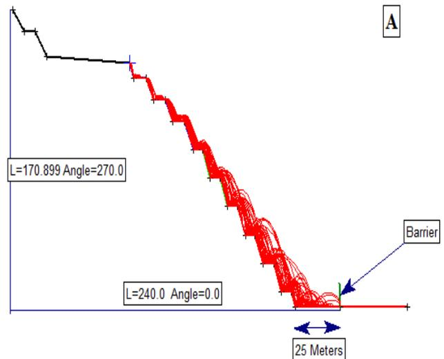
Fig. 10 Simulated horizontal location of rockfall end-points utilising a perfectly inelastic barrier located 25 meters from the slope toe.
