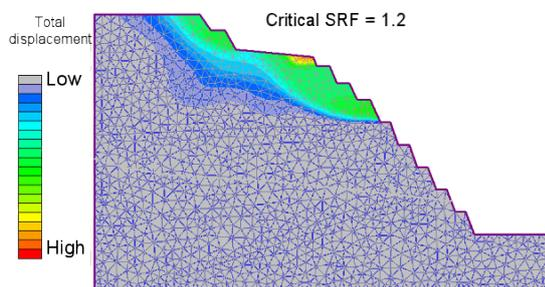
Fig. 6 The total displacement in the slope. The most critical displacement for the slope surface on which the proposed rocks could be detached, is located in the bottom of the ramp and nearby the upper benches around the haulage road.
