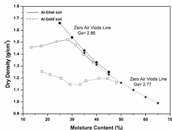
Fig. 4 Compaction curves of Al-Ghat and Al-Qatif soils
