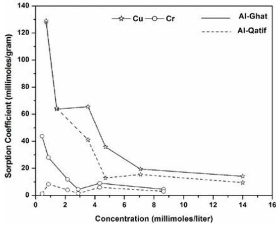
Fig. 7 Variation of sorption coefficient at different dilution ratios
