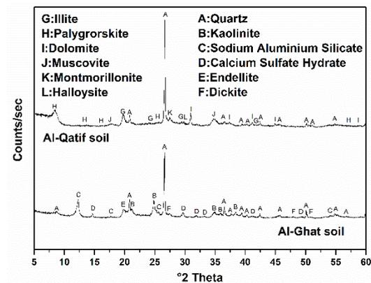
Fig.2 X-ray diffraction analysis
