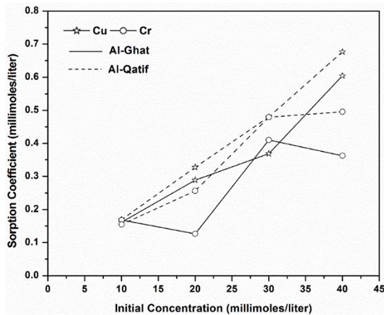
Fig. 8 Variation of sorption coefficient at various initial concentrations
