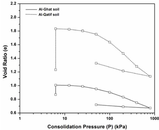
Fig. 5 Void ratio – pressure curves of Al-Ghat and Al-Qatif soils
