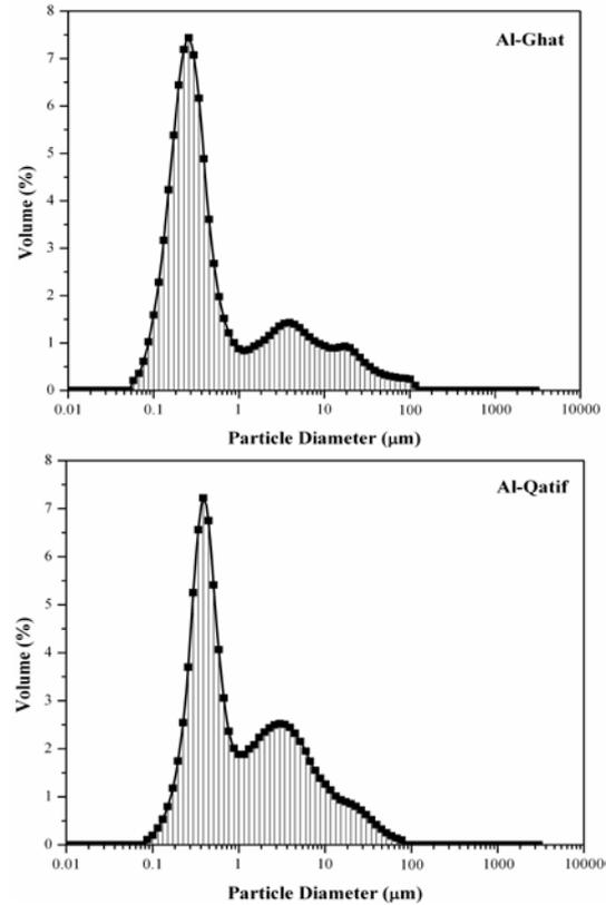
Fig.1 Particle size distribution curves
