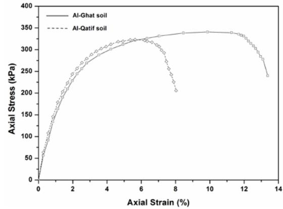
Fig. 6 Unconfined compression strength behavior of Al-Ghat and Al-Qatif soils
