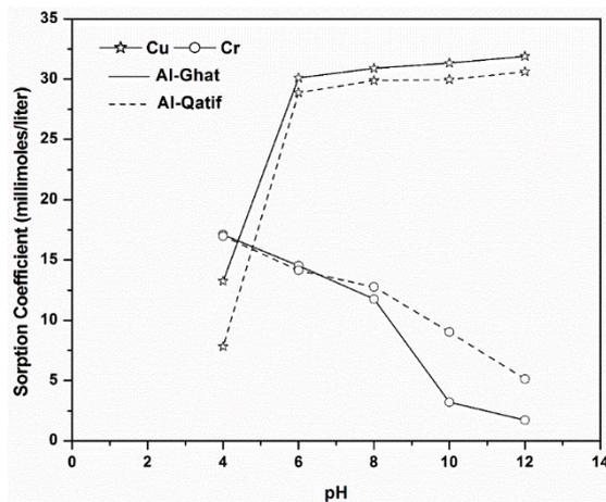
Fig. 9 Variation of sorption coefficient with pH
