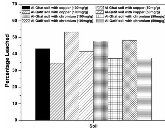
Fig. 10 Leaching behavior of selected soils for the targeted metal ions
