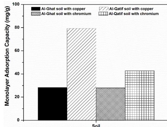
Fig. 11 Variation of monolayer adsorption capacity of selected soils for copper and chromium
