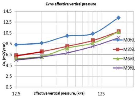
Figure 7 Effect of lime-treated marine clay on coefficient of consolidation ( $c_v$ ) at 28 curing days
