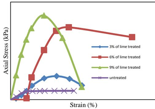
Figure 3 Axial stress versus Strain at 28 days
