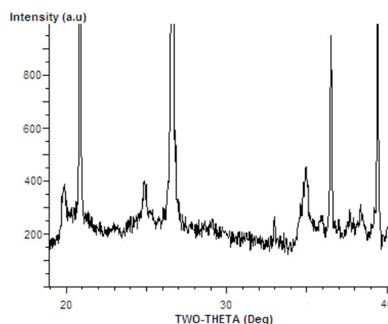
Figure 1 XRD pattern for the marine clay
