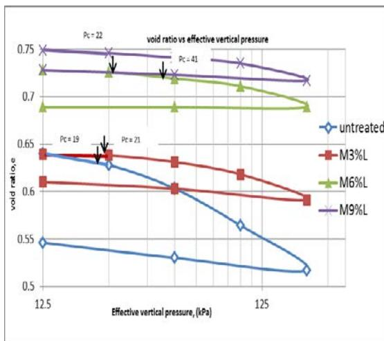
Figure 4 Effect of lime on compression curves of treated marine clay after 7 curing days
