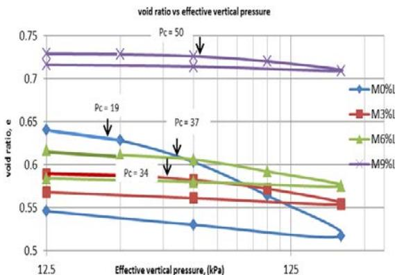
Figure 5 Effect of lime on compression curves of treated marine clay after 28 curing days
