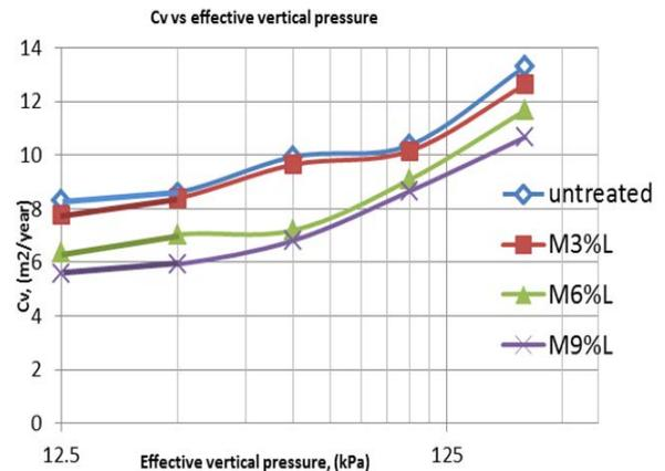
Figure 6 Effect of lime-treated marine clay on coefficient of consolidation ( $c_v$ ) at 7 curing days.
