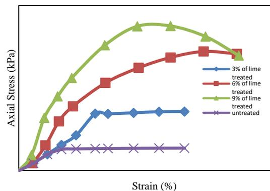
Figure 2 Axial stress versus Strain at 7 days
