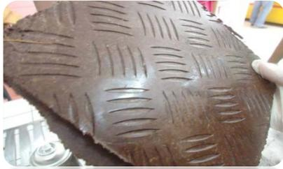
Fig. 3: The finished HDB product with wood tile quality.
