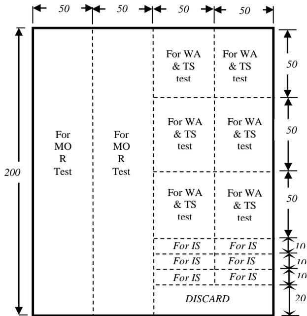
Fig. 4: Cutting pattern of test specimens for physical and mechanical testing (dimensions in mm.)
