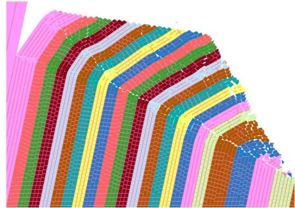
a) Block toppling, uphill scarp depth = 106.3 m, rupture surface at 28°
