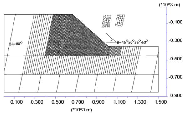
Fig. 2 Illustration of the numerical model geometry and joints details inside the beds
