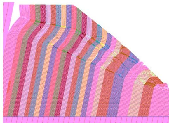
b) Multiple block toppling, 0.0085 bed-height (25 seconds)
