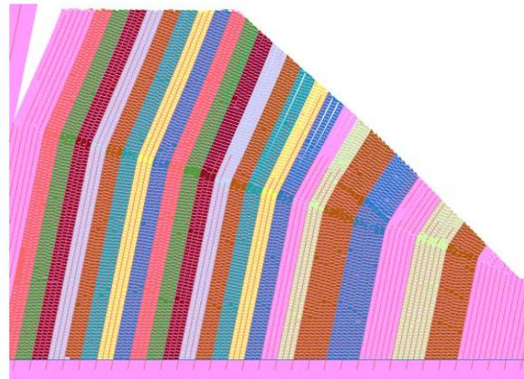
a) Block-flexural toppling, 0.017 bed height (25 seconds)
