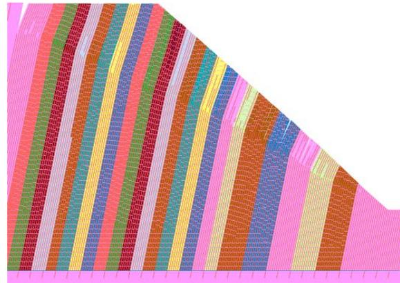
a) Block-flexural toppling, 40,000 cycles
