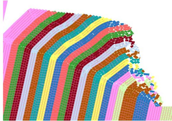
Fig. 7 Rock falls at 60° slope face angle and 0.017 bed-height ratio
