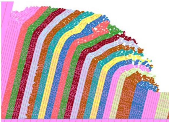
Fig. 9: Block toppling and rock falls, 60°slope, and 0.017 bed-height ratio at 720,000 cycles
