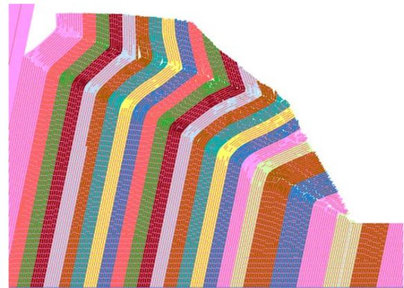
b) Multiple block toppling, uphill scarp depth = 83.8 m, rupture surface at 31°
