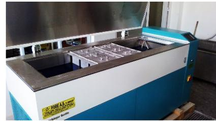
Fig. 4 CDF/CIF freezing thawing machine
