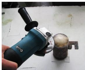
Fig. 3 Surface levelling of expanded part
