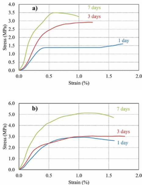
Fig. 7 Stress - strain behavior of frozen granular specimens, a. Poorly graded gravel, b. Poorly graded sand
