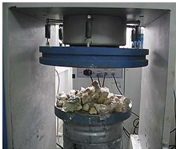
Fig. 10 Bursting formation under fast loading rate
