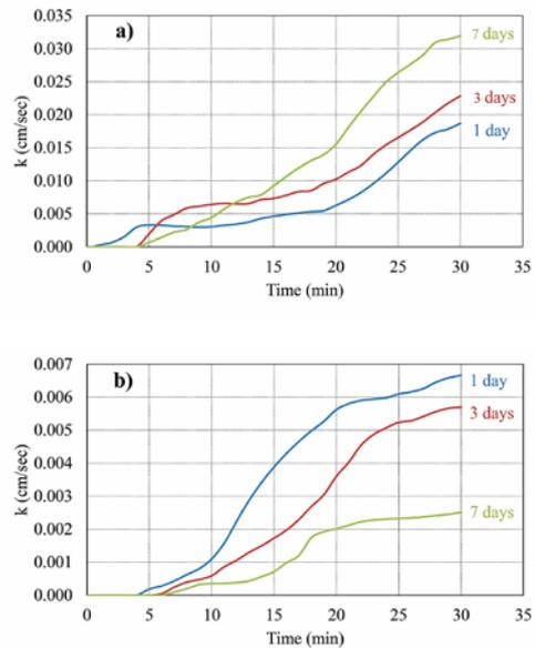
Fig. 8 Change in coefficient of permeability for frozen granular specimens, a. Poorly graded gravel, b. Poorly graded sand
