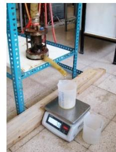
Fig. 6 Permeability test device
