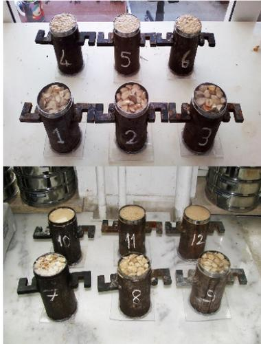
Fig. 2 Unfrozen gravel and sand specimens
