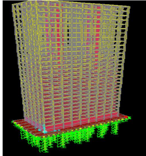
Fig:1 25 storey building supported on piled raft foundation
