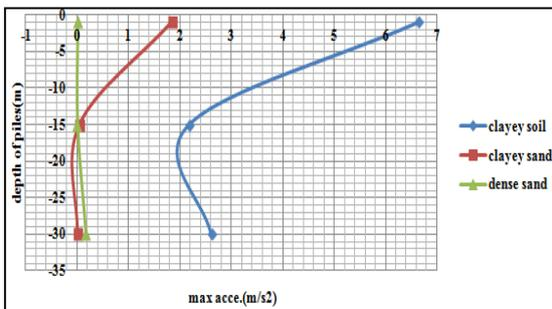
Fig: 8 Maximum acceleration for Bhuj earthquake. l = 30 m
