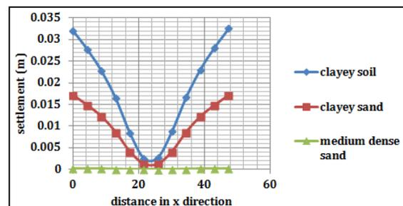
Fig: 4 Settlement of raft in z direction for El Centro earth quake (l = 15 m)
