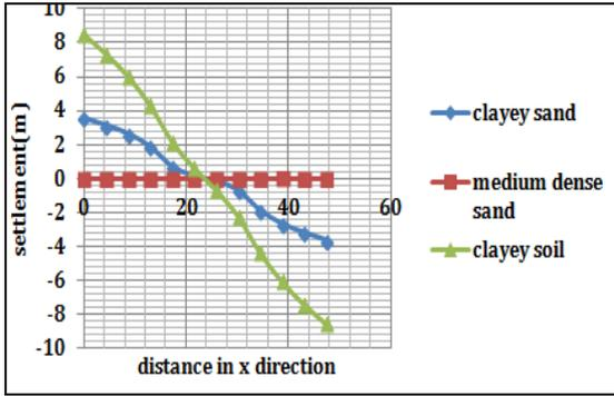
Fig: 5 For bhuj earthquake settlement in z direction (l = 30 m)
