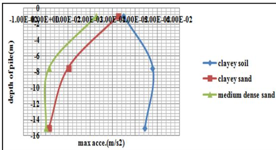
Fig:7 Maximum acceleration for El Centro earthquake. l = 15 m
