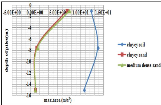
Fig: 6 Maximum acceleration for bhuj earthquake. l = 15 m
