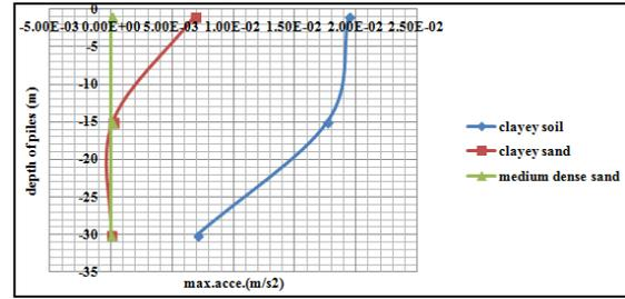
Fig: - 9 Maximum acceleration for El Centro earthquake. l = 30 m
