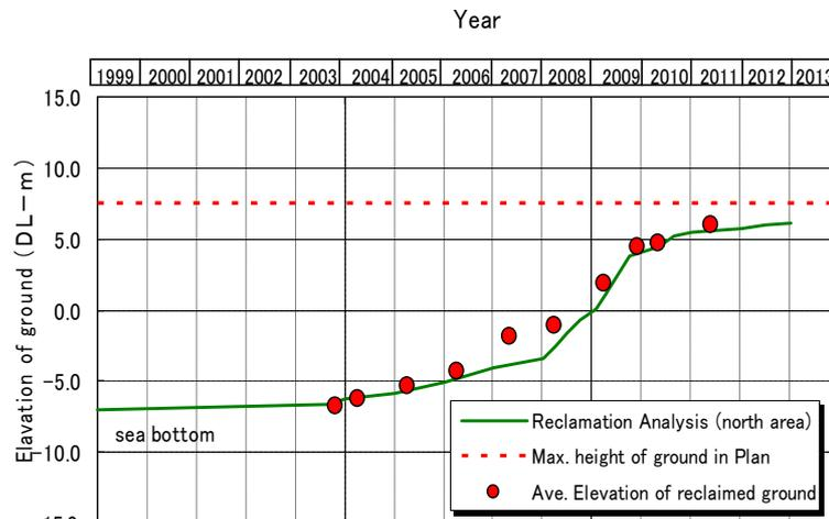
Fig. 12 Measured data and reclamation analysis result in the north area
