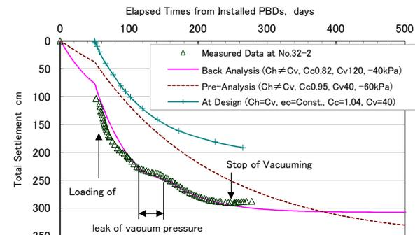
Fig. 6 Monitoring result and pre- and back- analyses
