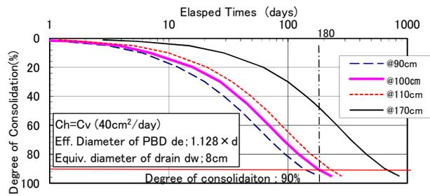
Fig. 11 Consolidation curves with different installation pitches and designed condition
