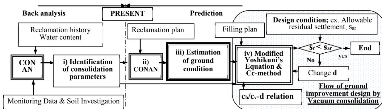
Fig. 15 Proposed design flow of vacuum consolidation for reclaimed ground with dredged clays
