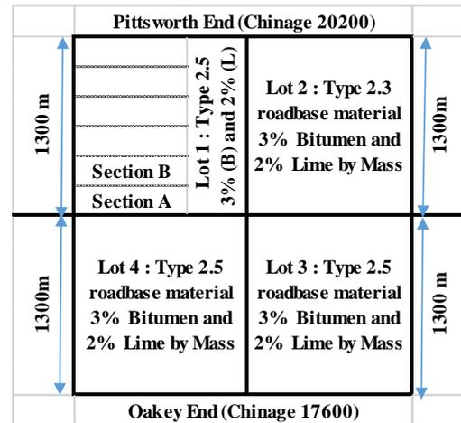
Fig.2 Site plan for segmental construction
