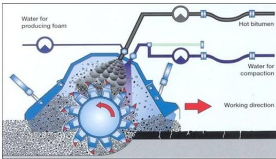
Fig.7 Foamed Bitumen mixing process [5]
