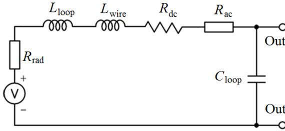
Fig. 4 Equivalent circuit of an inductive loop antenna
