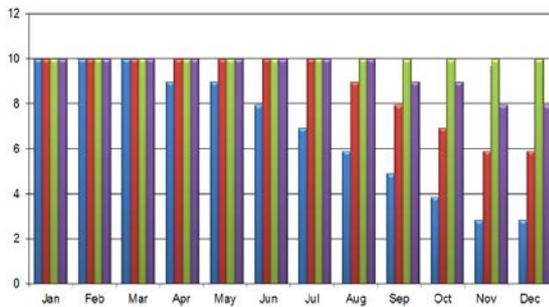
Fig. 10 Relation between scour and number of RFID tags
