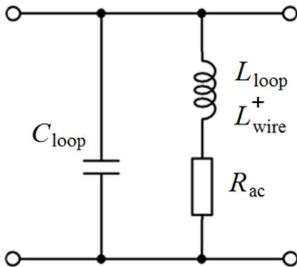
Fig. 6 Final equivalent circuit of the loop antenna
