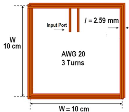
Fig. 5 Physical dimension of the loop antenna
