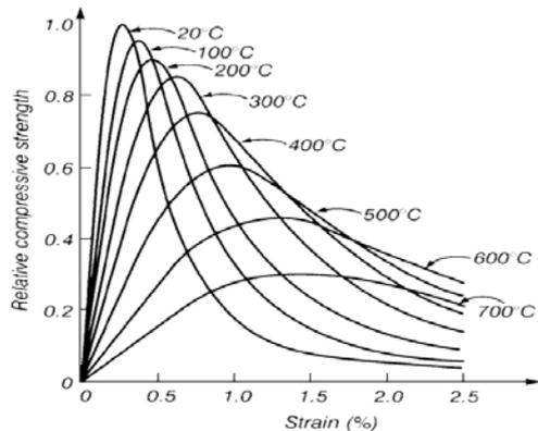
Fig. 7 Concrete stress-strain relationship at high temperature [30]
