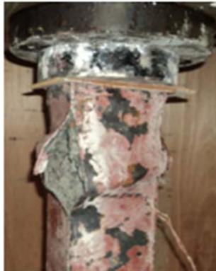
Fig. 4 Failure mode of ST strengthen columns [20]
