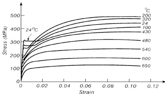
Fig. 8 Steel-strain relationship at high temperature [30]
