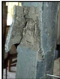
Fig.5 Failure mode of CFRP strengthen columns [20]
