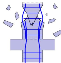
Fig. 2 Mechanism for mode of failure of RC column [1]-[2]
