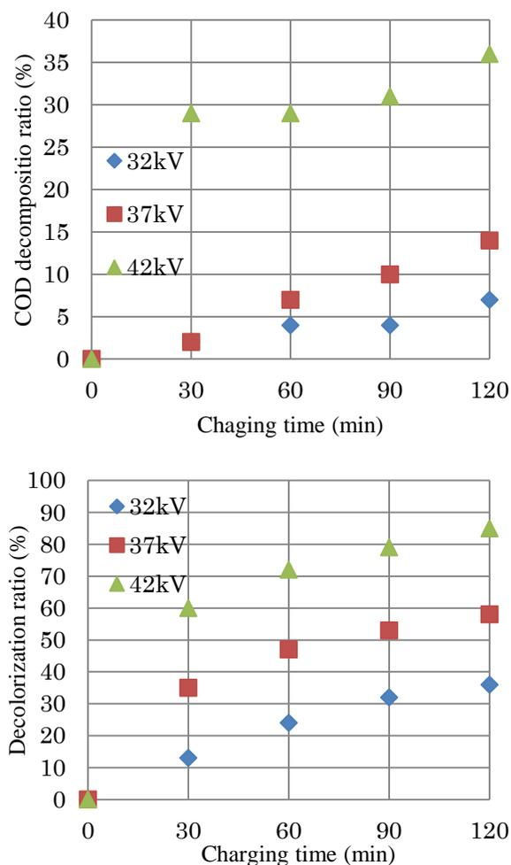
Fig.3 Effect of charging voltage on the ratios of COD decomposition and decolorization
