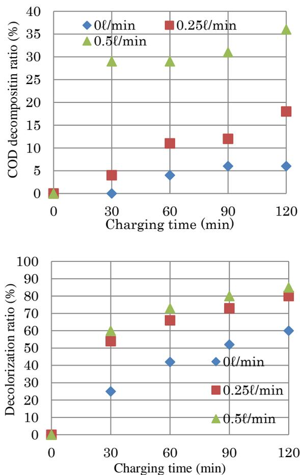
Fig.5 Effect of O<sub>2</sub> coexistence on the ratios of COD decomposition and decolorization
