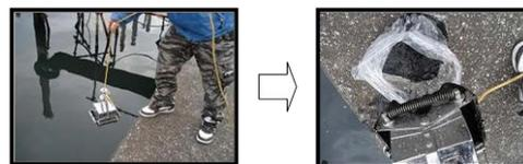
Fig.5 Scene of Catching Sludge.
