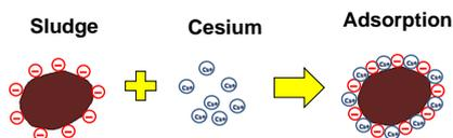
Fig.2 Mechanism on Adsorption of Cesium.
