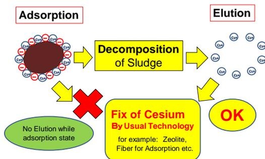
Fig.3 Mechanism on Fixing of Cesium from
