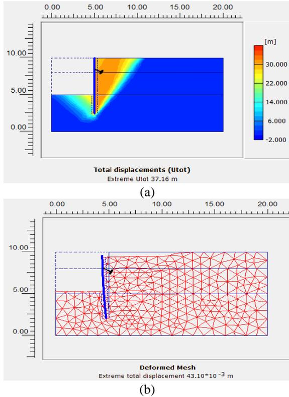
Fig. 6 Model results validated by PLAXIS software (a) total displacements and (b) deformed mesh
