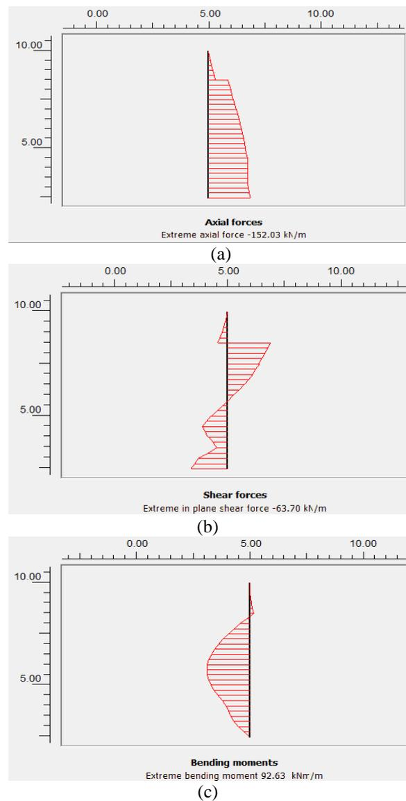
Fig. 5 Model results validated by PLAXIS software (a) axial forces, (b) shear forces and (c) bending moments
