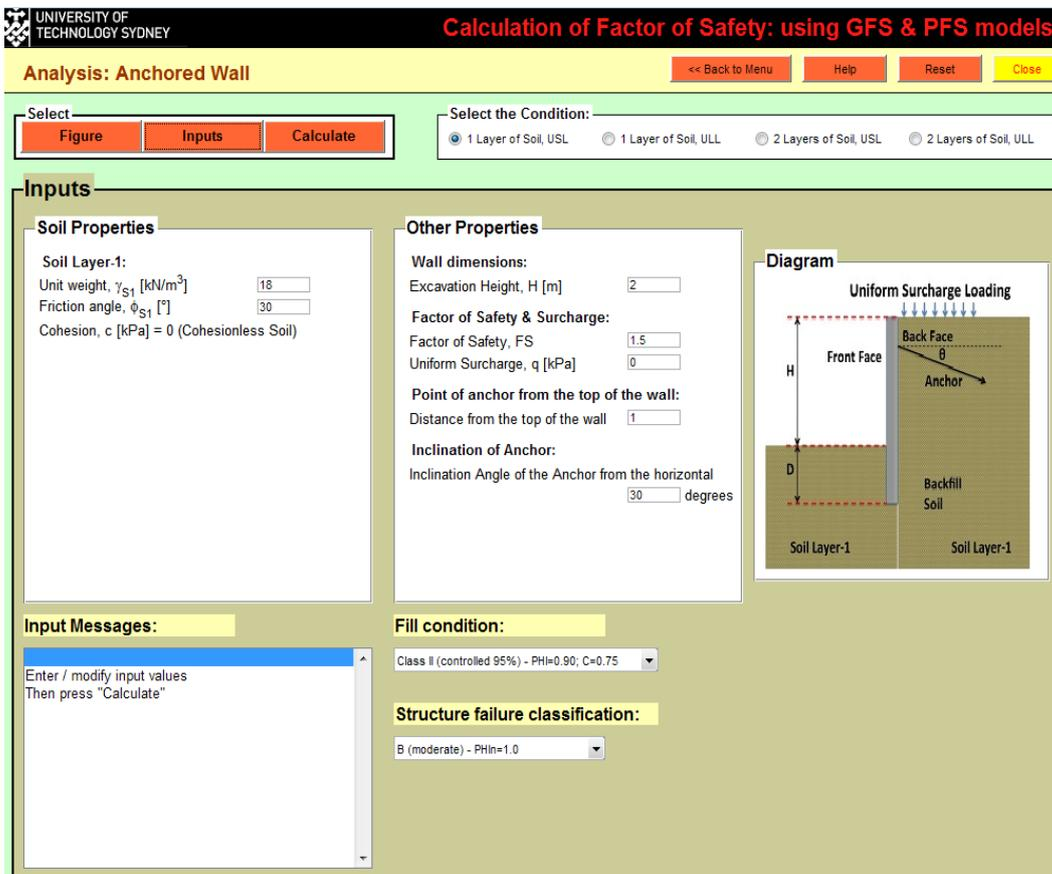
Fig. 3 A snapshot of the "Inputs" page of the model for an anchored wall
