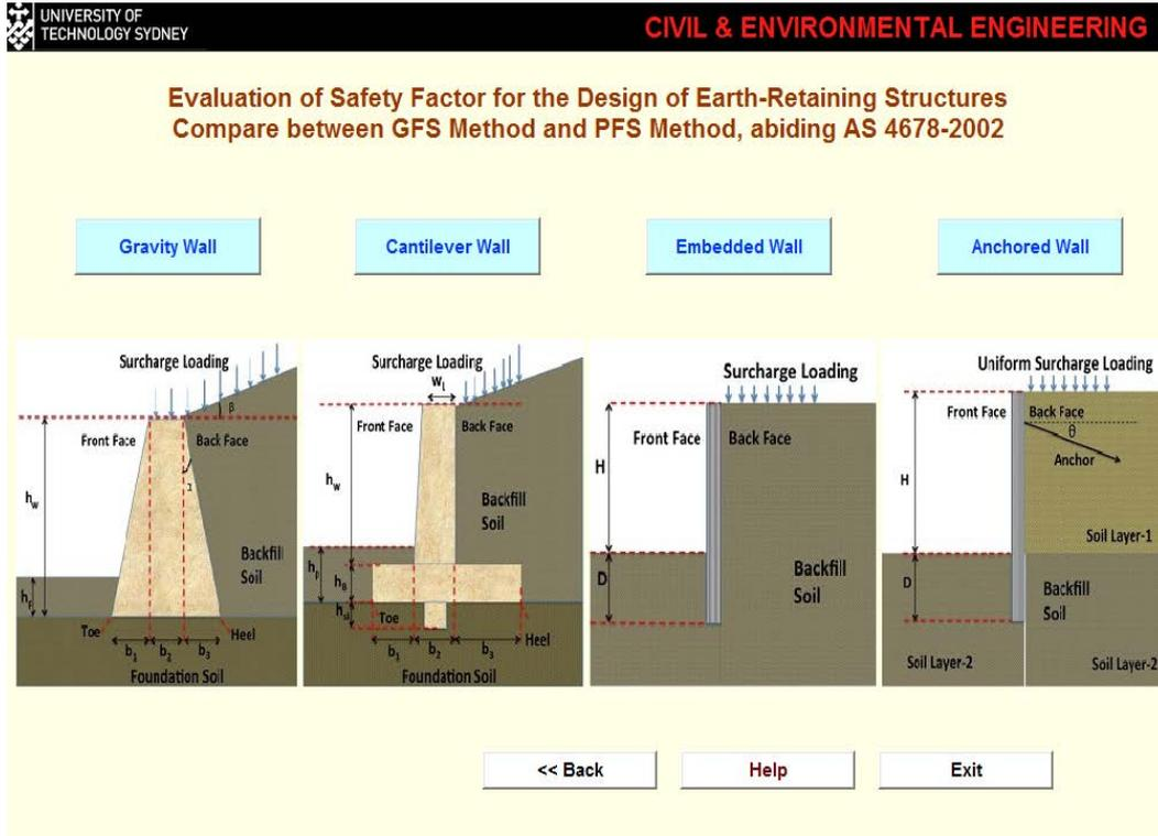
Fig. 2 A snapshot of the main page of the developed model using the graphical user interface in MATLAB
