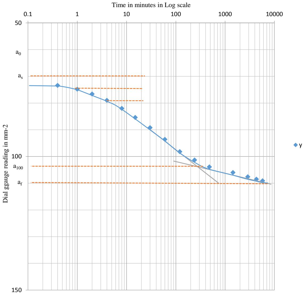
Fig. 3 SMSW Compression curve using Cassagrande's method
