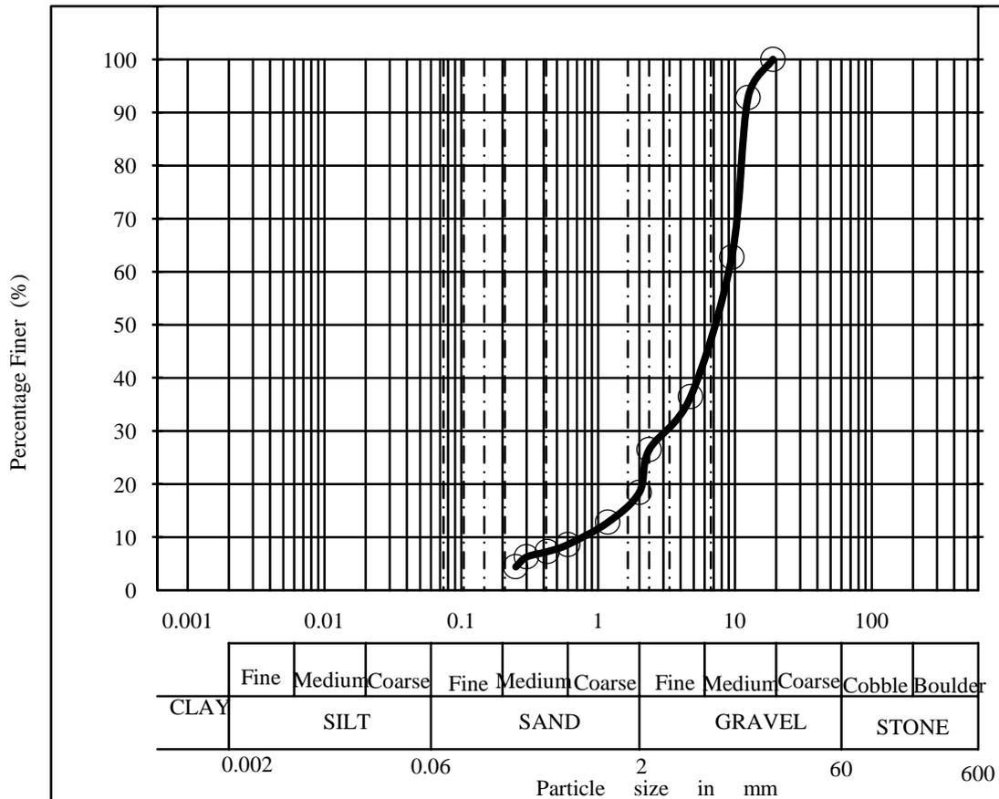
Fig. 1 SMSW particle size distribution curve
