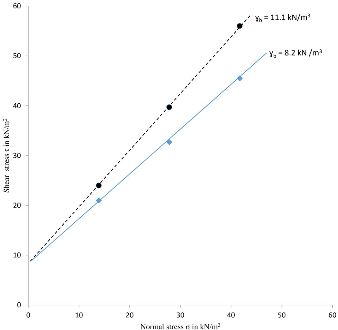
Fig. 4 SMSW shear strength failure envelope
