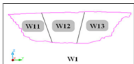
Fig.3 Subdivision outline of W1 slope of the pit into three vertical slices to study each slice (wall) with its own discontinuities.
