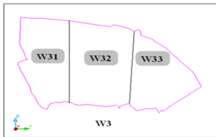
Fig.11 Subdivision outline to W3 slope element of the pit into three vertical slices to study each slice with its own discontinuities.
