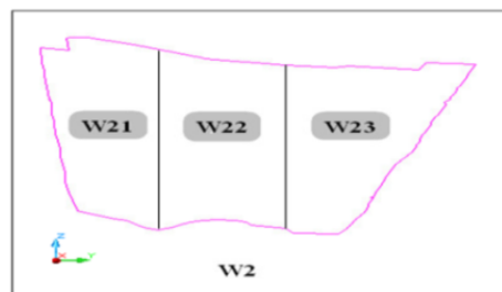
Fig.7 Subdivision outline to W2 slope element of the pit into three vertical slices to study each slice within the slope with its own discontinuities.
