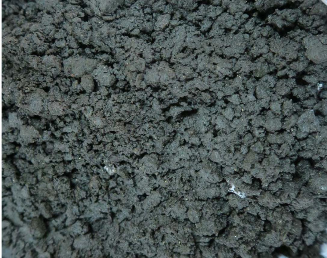
Fig. 2 Ready Mix Lawele Granular Asphalt (Scale 1:3)
