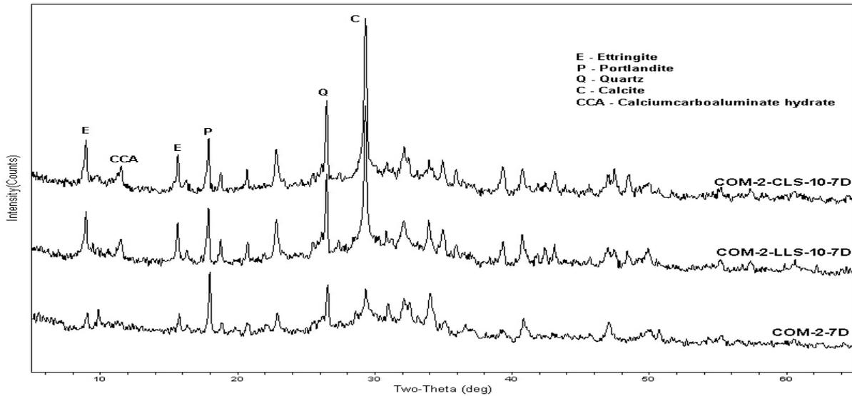
Fig.1 XRD of hydrated pastes of control cement COM-2 and multi blend cement samples containing low and cement grade limestone at 7 days
