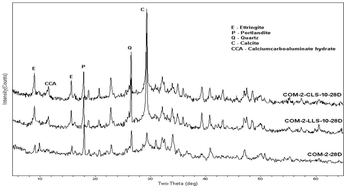
Fig.2 XRD of hydrated pastes of control cement COM-2 and multi blend cement samples containing low and cement grade limestone at 28 days
