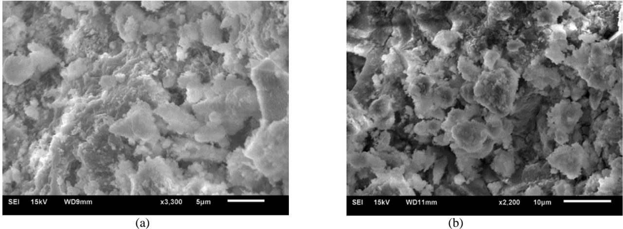
Fig.3 SEM images of 28 day hydrated multi blend cement containing (a) low-grade limestone and (b) cement-grade limestone
