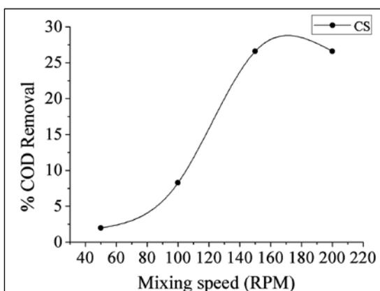
Fig.1 COD removal at 50,100, 150 and 200 shaking speeds
