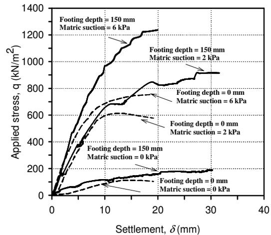
Fig. 4 Relationship between the applied stress versus settlement behavior of surface and embedded model footing tests (PLTs) of 150 mm × 150 mm using the UOBCE and the modified UOBCE.
