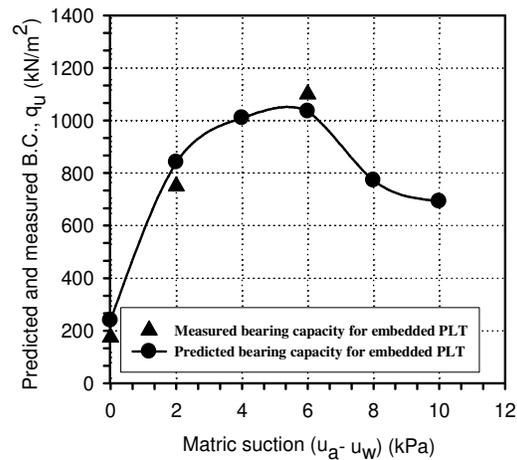
Fig. 8 Comparison between the predicted and measured bearing capacity for embedded model footing (PLT) of 150 mm × 150 mm in the modified UOBCE.
