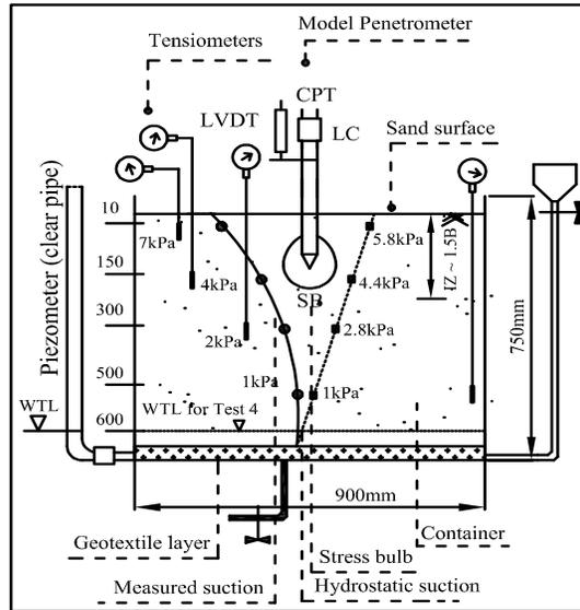
Fig. 5 Schematic to illustrate the procedure used for estimating the average matric suction of 6 kPa within the influence zone (IZ) in the UOBCE.
