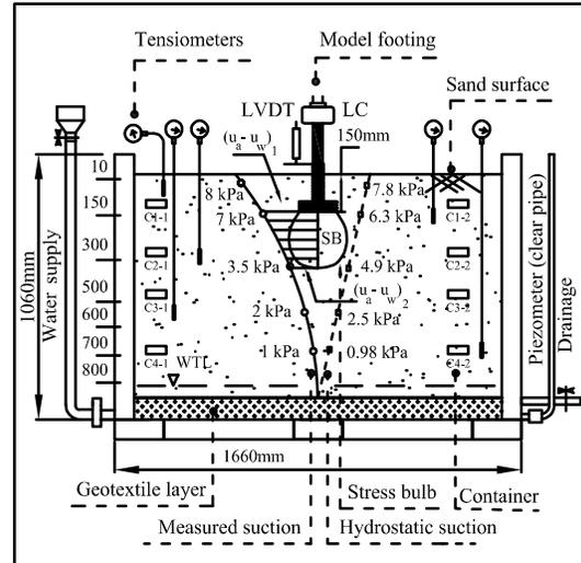
Fig. 3 Sectional view of the modified UOBCE test box with the average matric suction of 6 kPa within the stress bulb zone of embedded footing.
