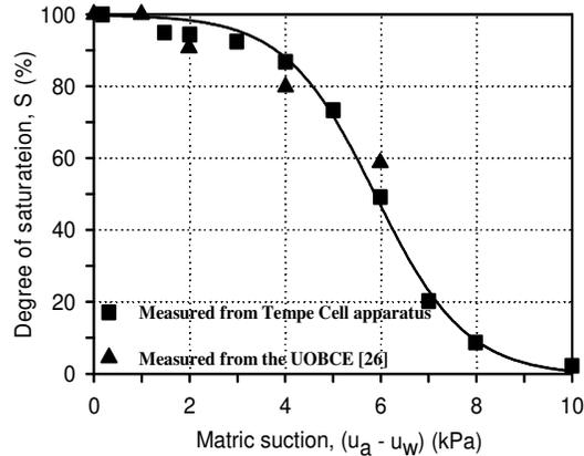
Fig. 6 Measured SWCC from the Tempe Cell apparatus and the test box of the UOBCE.
