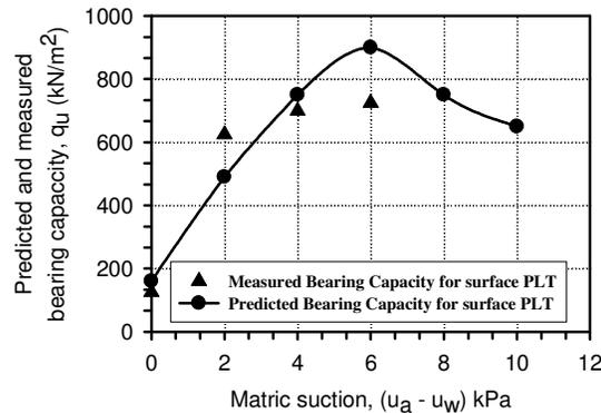
Fig. 7 Comparison between the predicted and measured bearing capacity of 150 mm × 150 mm surface model footing (PLT) in the UOBCE.
