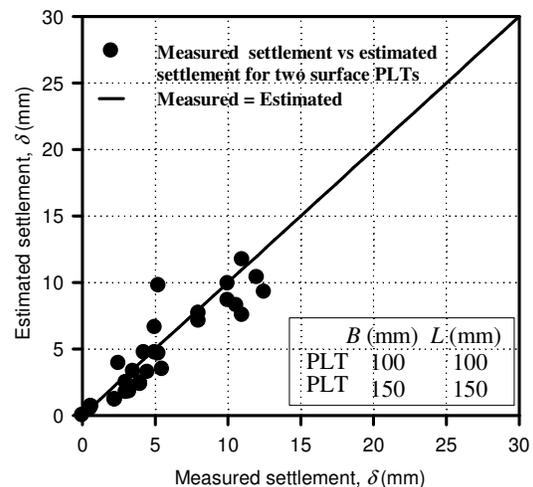
Fig. 9 Comparison between the measured settlements for two surface model footings (PLTs) carried out in the UOBCE and the estimated values using modified Schmertmann's equation.
