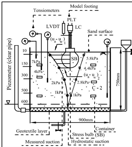
Fig. 2 Schematic to illustrate the procedure used for estimating the average matric suction of 6 kPa within the stress bulb zone of surface footing.
