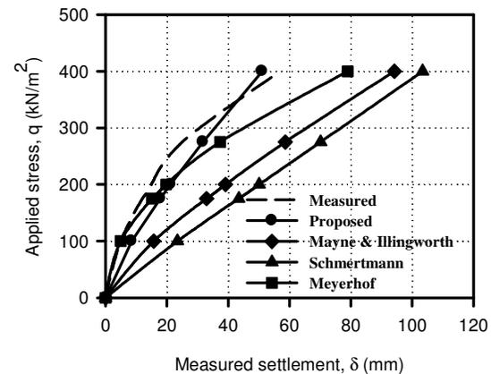
Fig. 10 Comparison between estimated and measured settlement using the modified Schmertmann's equation for a large-scale footing (i.e., FLT of 1500 mm × 1500 mm from [32]).
