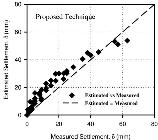
Fig. 11 Comparison between estimated and measured settlements of seven large-scale footing load tests (four FLT's from [32] and three FLT's from [34]) using the modified Schmertmann's equation.
