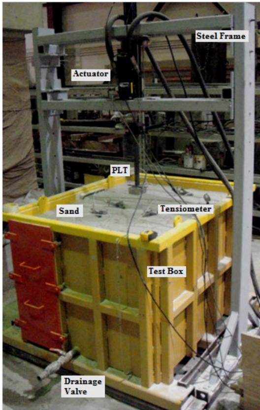
Fig. 1 Modified University of Ottawa bearing capacity equipment (modified UOBCE).
