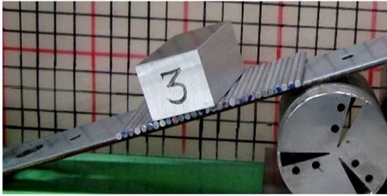
Fig. 3 Outline of the sliding test used to measure friction coefficient between model ground and modular-block.
