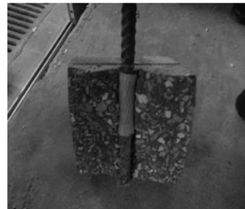
Fig.11: 16 mm re-bars splitting behavior.
