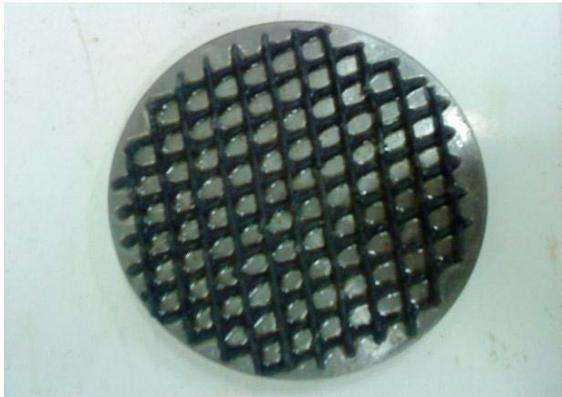
Fig. 3 Rough base of Circular footing.
