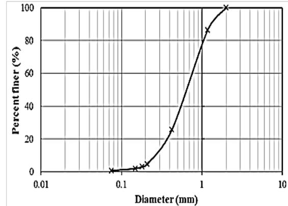
Fig. 1 Grain size distribution curve of sand.
