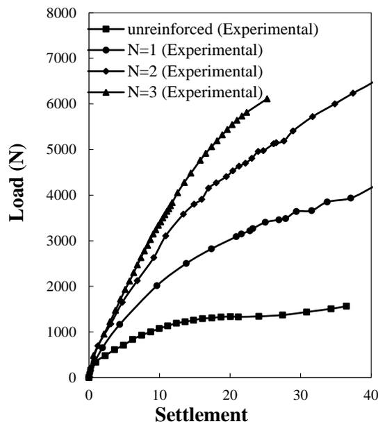
Fig. 7 Load versus settlement for reinforced and unreinforced sand for circular footing.
