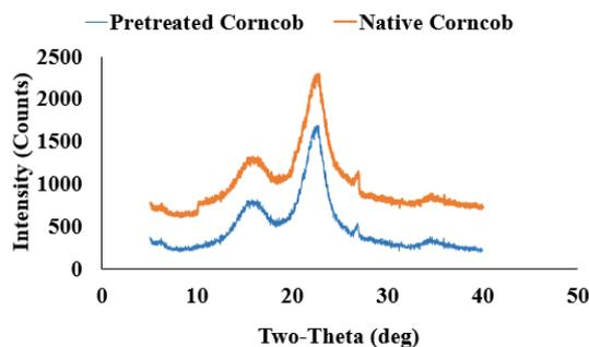
Fig. 5 X-ray diffraction profiles of the native (-) and pretreated biomass (-)
