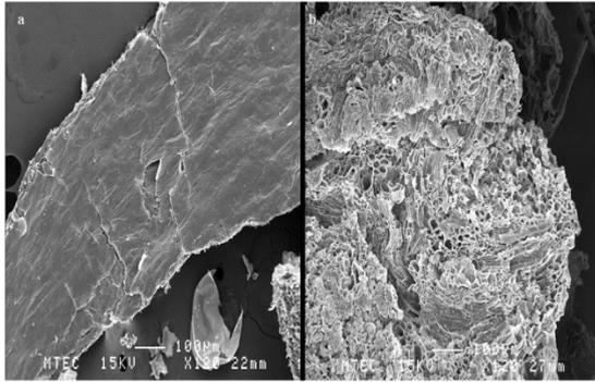
Fig. 4 X- Scanning electron micrographs of native and solid residues from pretreatment of corn cob under optimal condition. (a) Native corn cob; (b) pretreated corn cob at 5% H<sub>2</sub>O<sub>2</sub> concentration at 60°C for 2 h.
