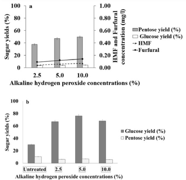
Fig. 1 Fig. 1 Effect of  $H_2O_2$  concentration on sugar releases into the liquid phase (a) sugar and inhibitory by-products (b) sugar after enzymatic hydrolysis
