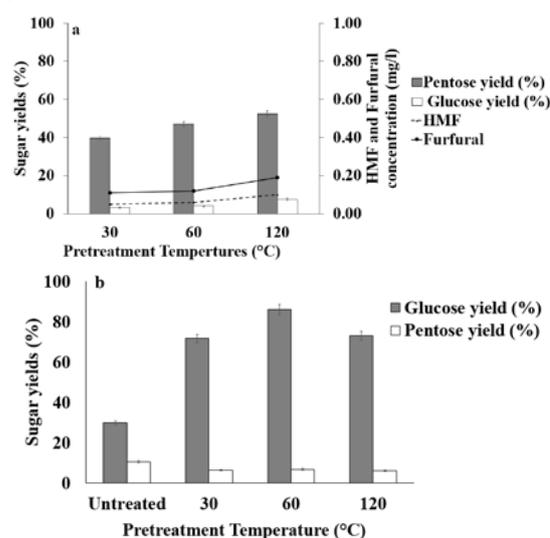
Fig. 2 Effect of pretreatment temperature on sugar releases into the liquid phase (a) sugar and inhibitory by-products in (b) sugar after enzymatic hydrolysis
