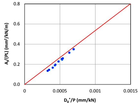
Fig.18 Relationship between the deflection area divided by the load value and the slab span length ( $A_v/PL$ ) and the assigned deflection at the loading point divided by the load value ( $D_0^*/P$ )
