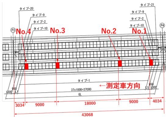
Fig.15 Positions of FWD measurements
