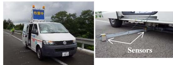
Fig.1 A vehicle equipped with the FWD testing machine
