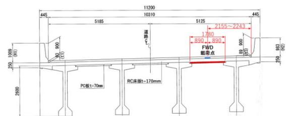
(c) Cross section of PCT composite bridge
