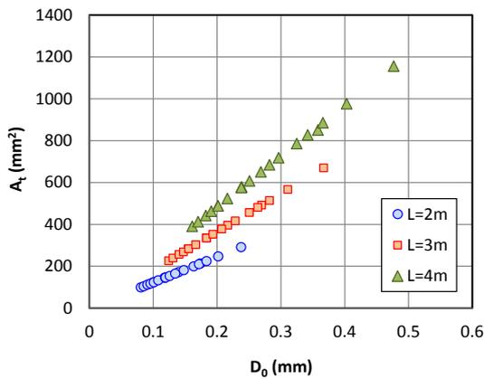
Fig.3 Relationship between the deflection area in the transverse direction ( $A_t$ ) and the deflection at the loading point ( $D_0$ )
