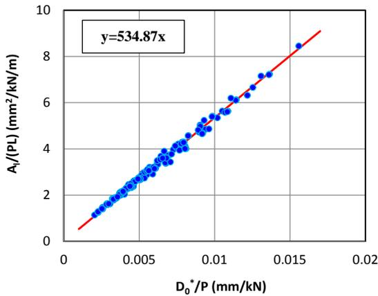
Fig. 11 The relationship between the deflection area divided by the load value and the slab span length ( $A_i/PL$ ) and the assigned deflection at the loading point divided by the load value ( $D_0^*/P$ )
