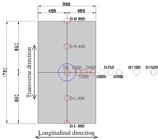
Fig.16 Loading position and deflection measuring points on PC panel
