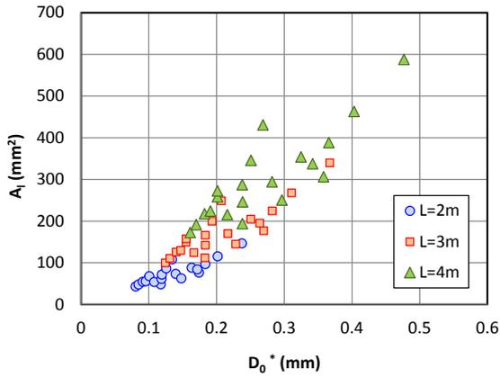
Fig.7 Relationship between the deflection area ( $A_l$ ) in the longitudinal direction and the assigned deflection at the loading point ( $D_0^*$ )
