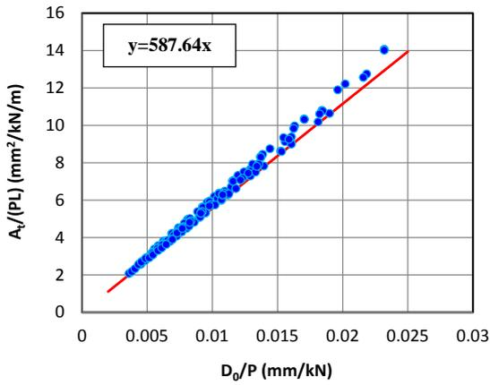
Fig.10 Relationship between the deflection area divided by the load value and the slab span length ( $A_i/PL$ ) and the deflection at the loading point divided by the load value ( $D_0/P$ )
