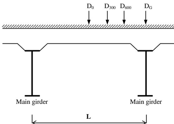
Fig.2 Arrangement of deflection measurement sensors in the transverse direction
