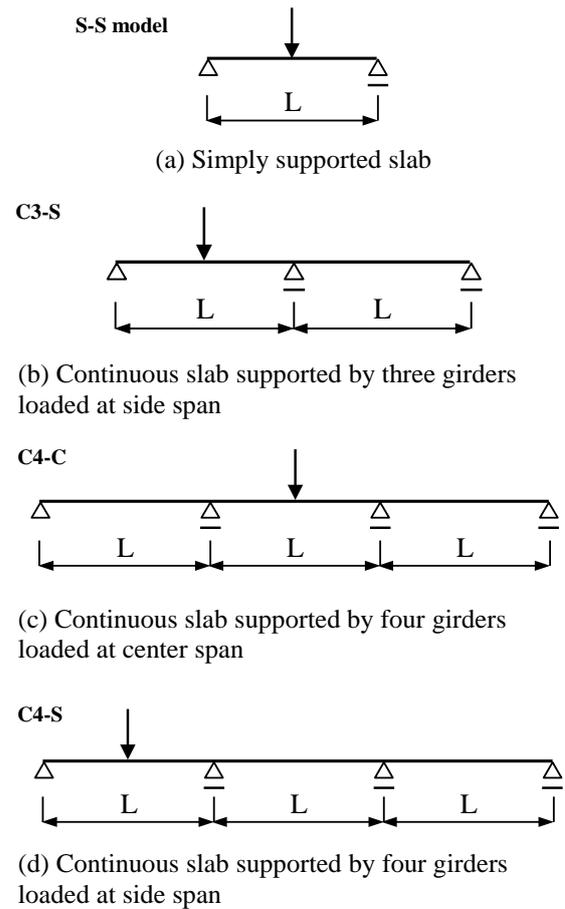
Fig. 9 Analytical models for continuously supported slabs
