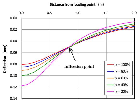
Fig.5 Deflection curves in the longitudinal direction of RC slabs (slab span length of 2 m) with several deteriorations
