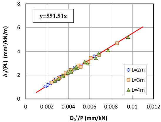
Fig.8 Relationship between the deflection area divided by the load value and the slab span length ( $A_l/PL$ ) and the assigned deflection at the loading point divided by the load value ( $D_0^*/P$ )
