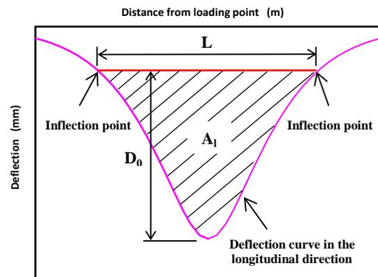
Fig.6 Deflection area in the longitudinal direction ( $A_l$ ) and the deflection at the loading point ( $D_0^*$ ) assigned to calculate between inflection points
