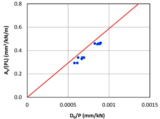
Fig.17 Relationship between the deflection area divided by the load value and the slab span length ( $A_v/PL$ ) and the deflection at the loading point divided by the load value ( $D_0/P$ )
