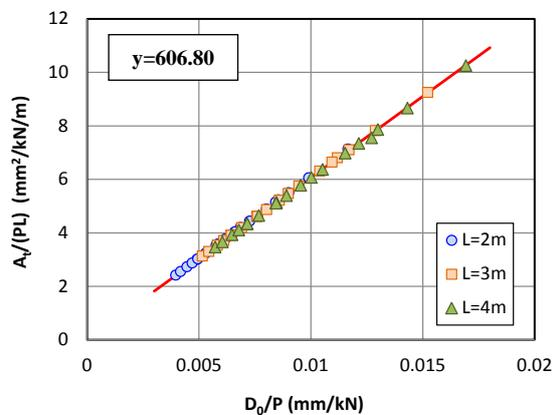
Fig.4 Relationship between the deflection area divided by the load value and the slab span length ( $A_t/PL$ ) and the deflection at the loading point divided by the load value ( $D_0/P$ )
