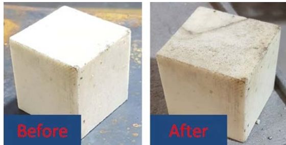
Fig. 3 Minor darkening of specimens at 72 °C after 836 hours
