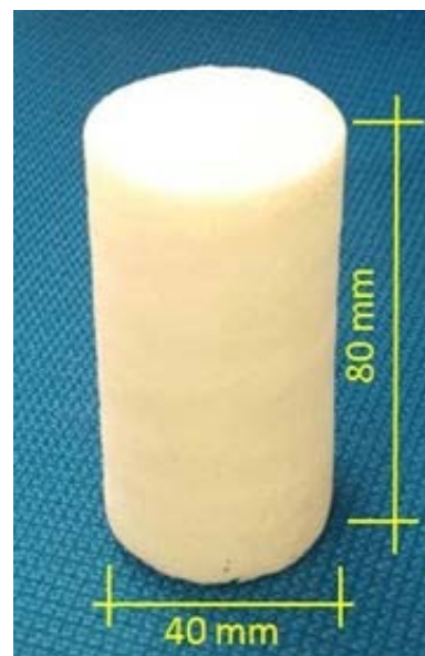
Fig.1 Obtained cylindrical specimens for a density test
