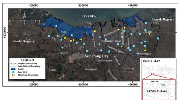
Fig. 2 Geophysical survey (yellow dots) and hydrogeological mapping points (blue dots).
