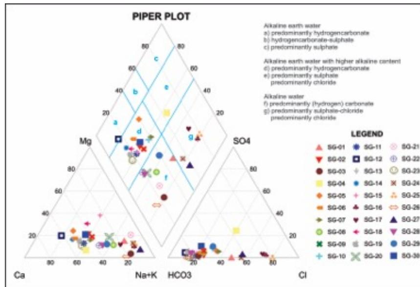
Fig. 5 Piper plot showing the groundwater facies.
