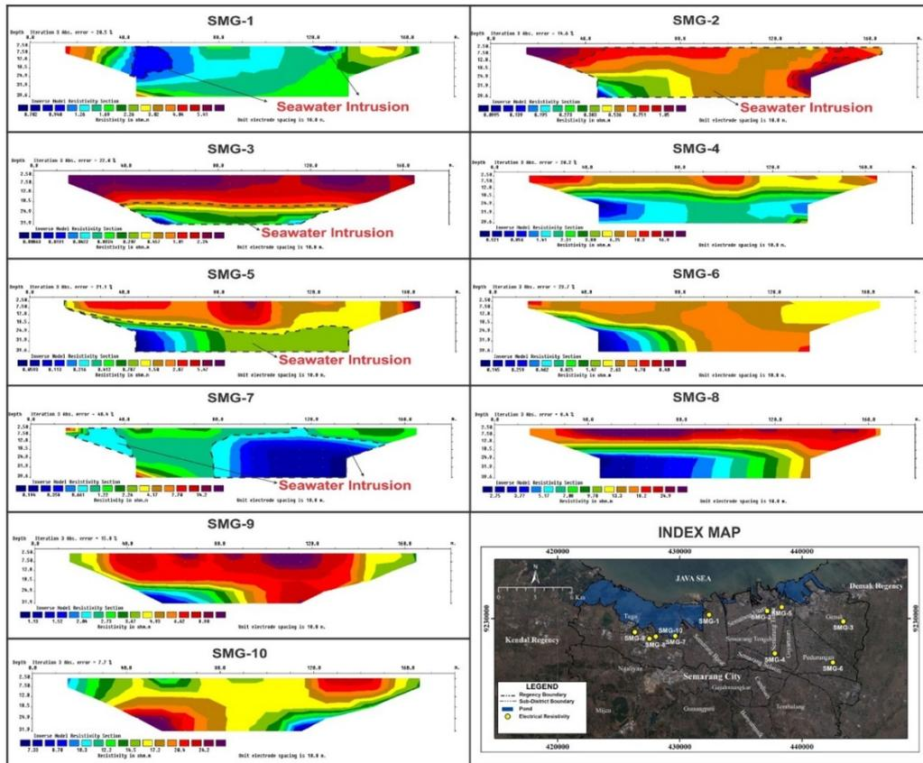
Fig. 3 Inverse model resistivity section of Geophysical survey.
