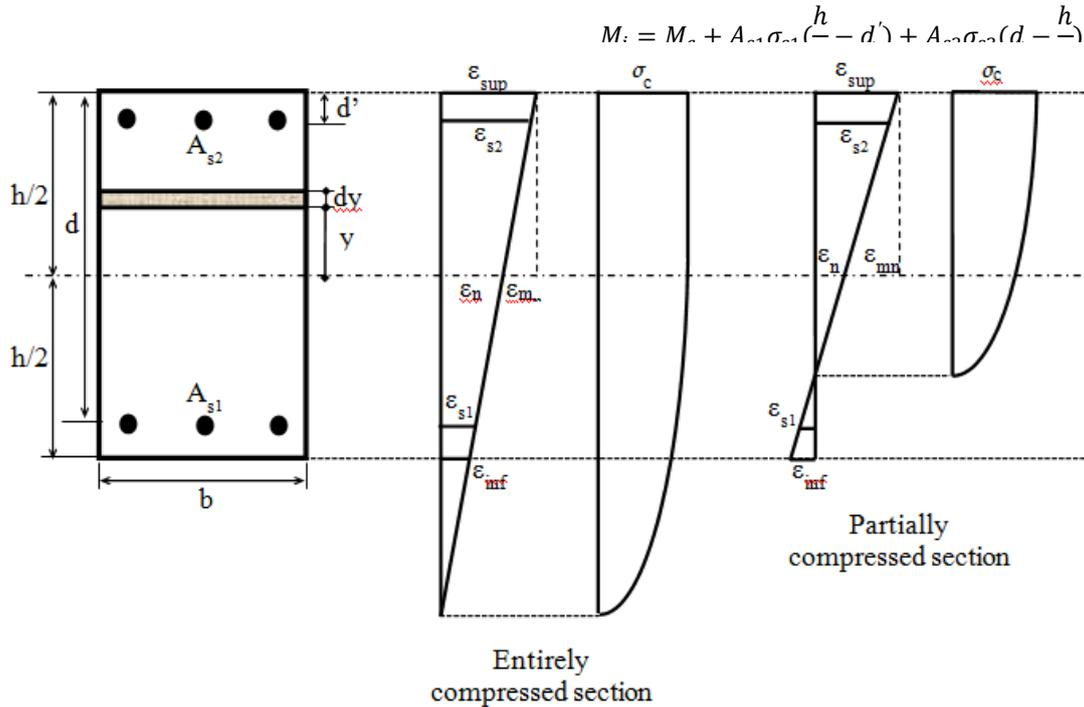
Fig.5: strains and stresses diagrams
