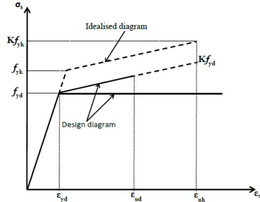
Fig.4: stress-strain diagrams for reinforcing steel
