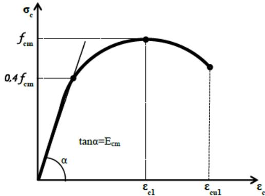
Fig.3: Stress-strain relation for concrete
