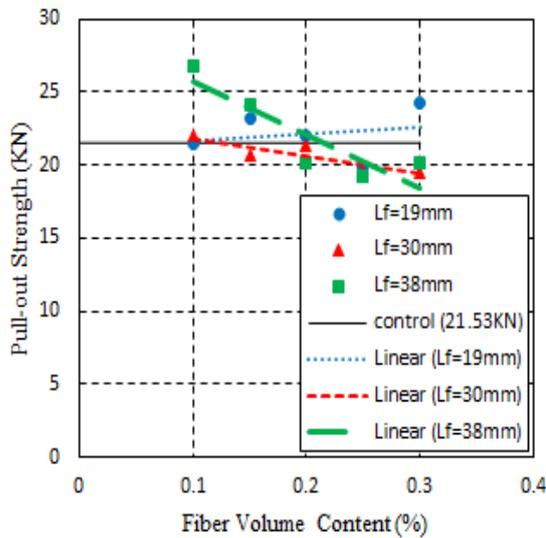
Fig. 5 Influence of fiber volume content to pull-out strength of CFRC
