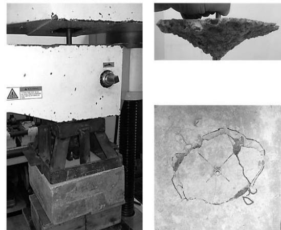
Fig. 2 Pull-out test set up and failure mode
