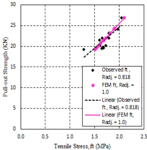
Fig. 8 Comparison of observed  $f_t$  and FEM  $f_t$
