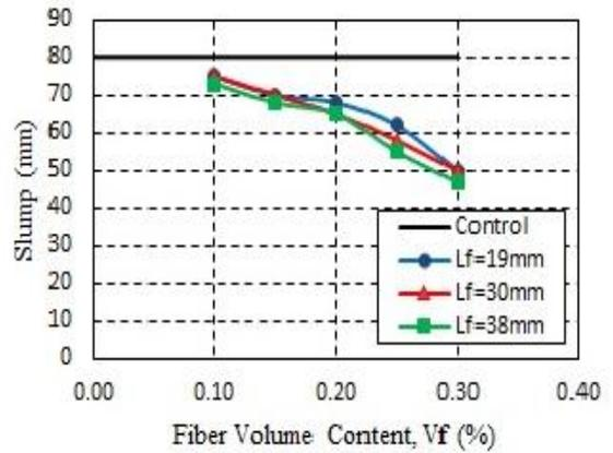
Fig. 4 Effect of fiber volume content to slump of CFRC mix
