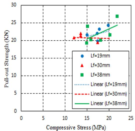
Fig. 6 Influence of compressive stress to pull-out strength of CFRC
