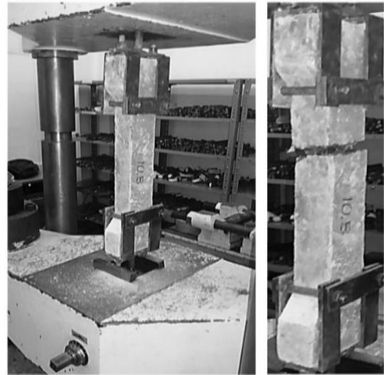
Fig. 1 Tension test set up and failure mode
