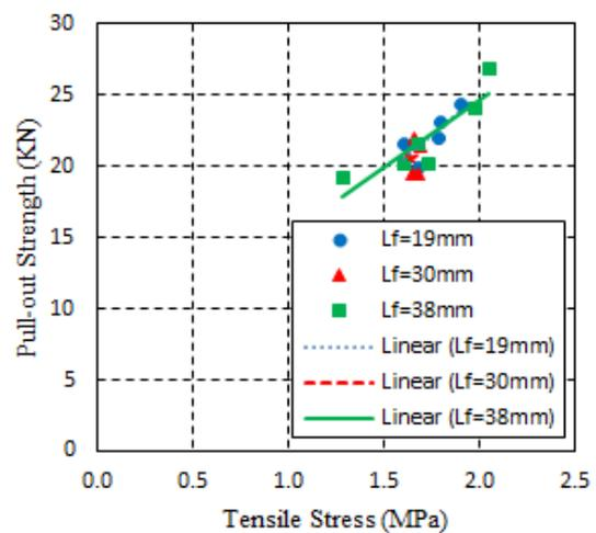
Fig. 7 Influence of tensile stress to pull-out strength of CFRC
