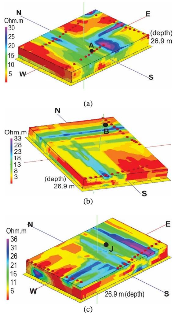
Fig.3 3D resistivity imaging from 2D resistivity imaging from lines located around (a) well A; (b) well B; (c) well J.
