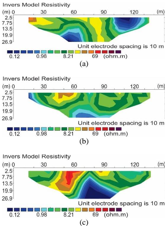
Fig.2 The 2D subsurface resistivity imaging of line
