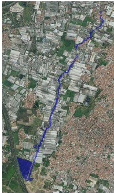
Fig. 16 Simulation with 315.000 m 3 Retention Pond for 2 year Return Period.
