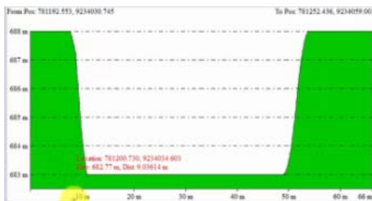
Fig. 13 Cross Section of 125 000 m 3 Retention Pond
