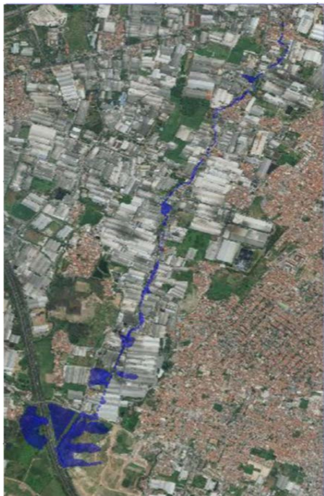
Fig. 14 Simulation with 125 000 m 3 Retention Pond for 2 year Return Period.
