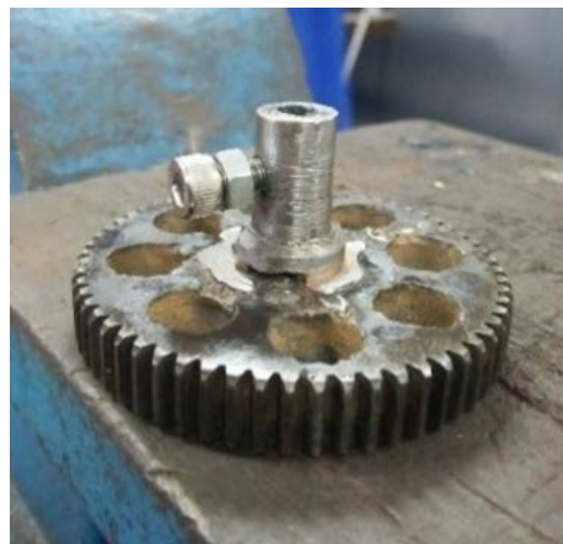
Fig.12 Gear as an ETC rotation transmission
