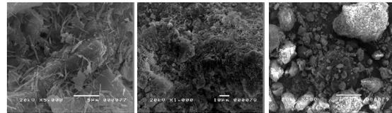
Fig. 1. Microfabric of 100S (5000x, 1000x and 500x Magnification)
