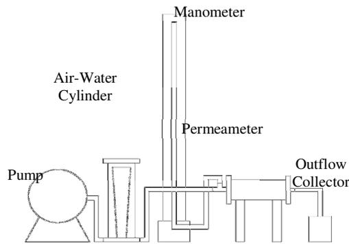
Fig. 1. Horizontal Permeability Set-up
