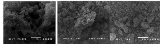
Fig. 2. Microfabric of 100FA (5000x, 1000x and 500x Magnification)
