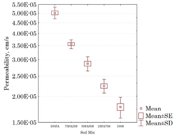
Fig. 4. Effect of fly ash on the vertical permeability when added to soil
