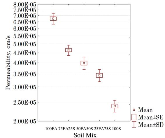
Fig. 5. Effect of fly ash on the horizontal permeability when added to soil
