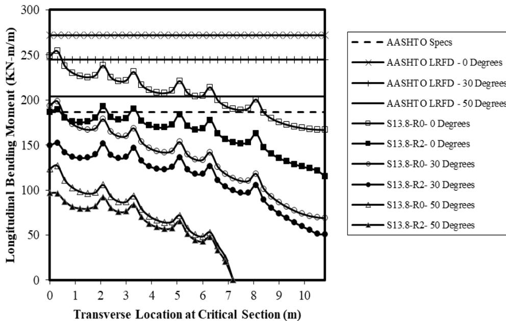
Fig. 4 FEA and AASHTO Standard (Specs) and LRFD moments for 13.8 m (46 ft) span, three-lane skewed bridges with railings and reference straight bridges without railing
