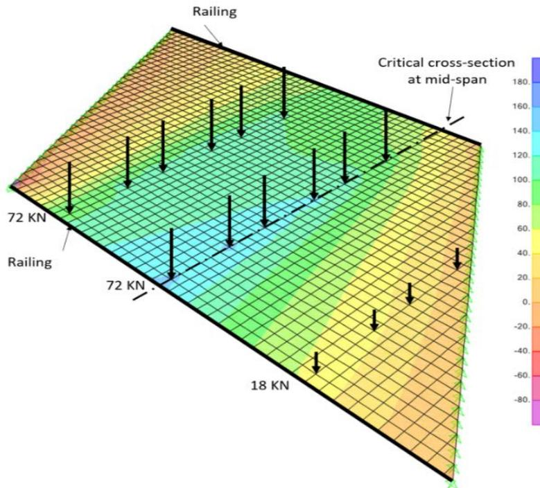
Fig. 3 FEA discretization and moments (KN-m/m) in a 13.8 m (46 ft) span, three-lane, 30° skewed bridge with railings, subject to HS20 Edge loading condition
