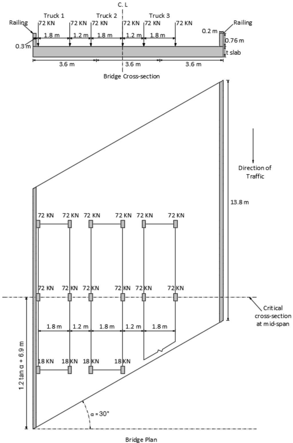
Fig. 2 Typical cross-section and layout for a 13.8 m (46 ft) span, three-lane, 30 degrees skewed bridge with railings, subject to HS20 Edge loading condition
