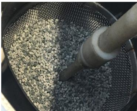
Fig.3 Stainless steel 2.5 mm sieve and point electrode
