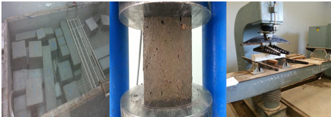
Fig.2 Cube and beam curing and testing of compressive and flexural strength
