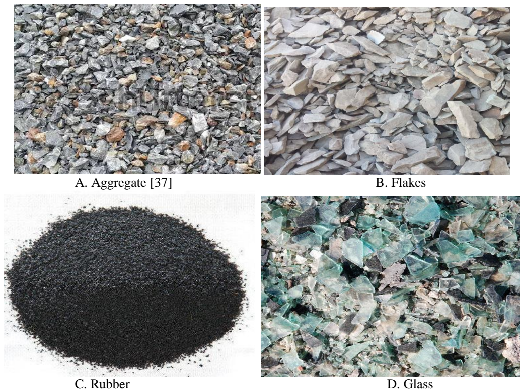
Fig.1 Recycled: A. aggregate, B. Flakes, C. Rubber, and D. Glass
