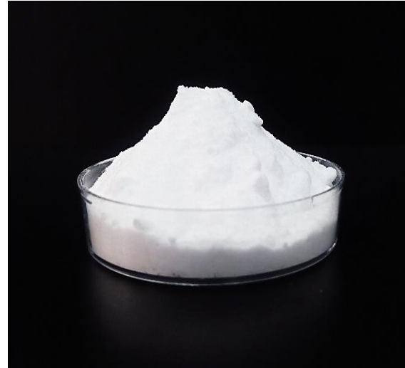
Fig.2 Powdered nanosilica synthesized from rice hull ash
