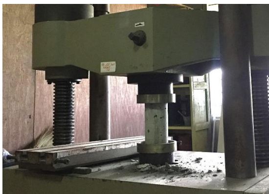
Fig.4 Compressive strength test setup
