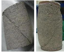
Fig. 2 Mode of failure for bottom ash.
