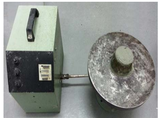
Fig. 2. Set-up of the flow table test.
