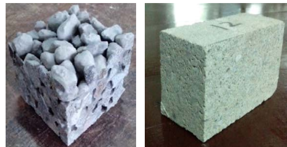
Fig. 6 Porous paving block (left) and normal paving block (right)
