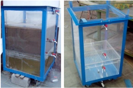
Fig. 5 Acrylic box for modeling of permeability test
