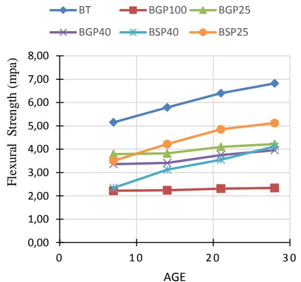
Fig 16 Flexural strength test with different amount of pozzolan (MPa)
