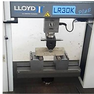
Fig. 15 Flexural strength test
