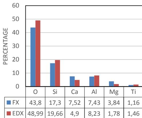
Fig. 12 Comparison of results fluorescence and SEM analysis
