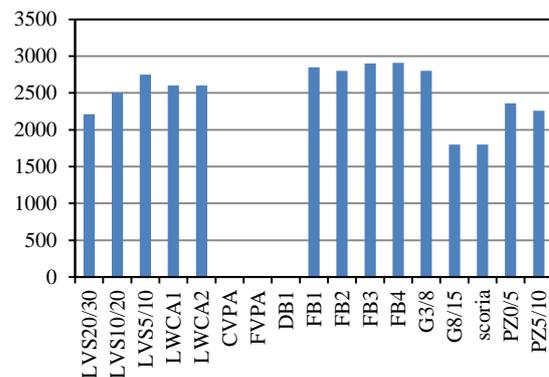
Fig. 5 Comparison of specific density of many pozzolans
