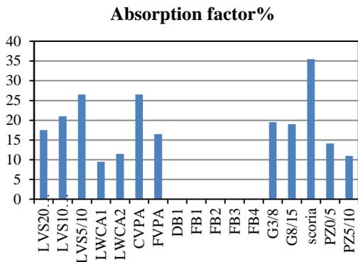
Fig. 6 Comparison of absorptions factors of different pozzolans
