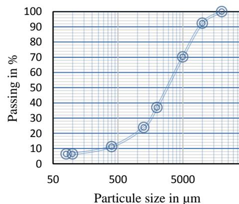
Fig.2 The granulometric curve of a sample of the pozzolan used
