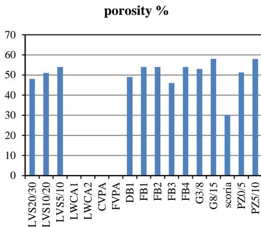
Fig.7 Comparison of porosity of different pozzolans
