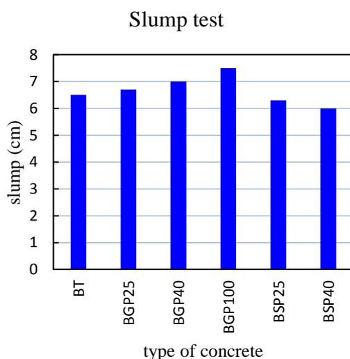
Fig. 13 Slump test with different amount of pozzolan
