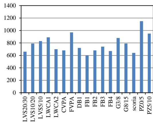
Fig. 4 Comparison of Bulk density of different pozzolans
