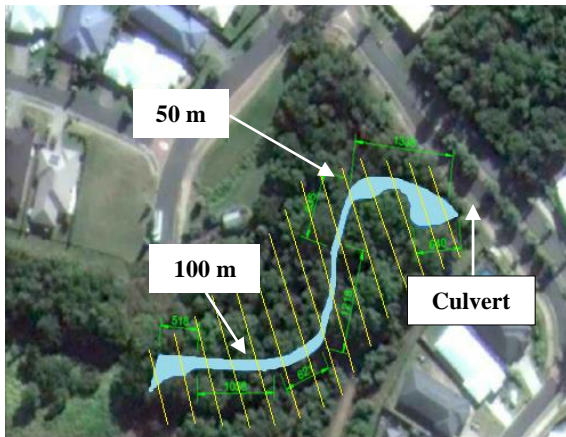
Figure 3: Real stream debris release distances (scaled in model); streambed and 50yr ARI flow area highlighted (hatched yellow)
