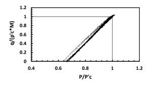
Fig.10. Critical state normalizing for the plain CDG soil under drained conditions.
