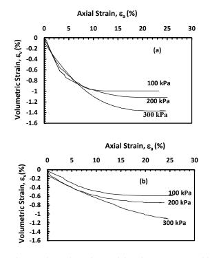
Fig. 5. Volumetric strain vs axial strain CID test: (a) with 10% fine sand, (b) with 40% fine sand.
