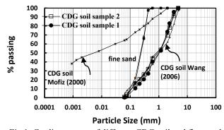
Fig.1. Grading curves of different CDG soil and fine sand samples
