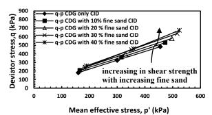
Fig. 6. Comparison between drained strength envelopes for CDG soil with different fine sand content of CID test.
