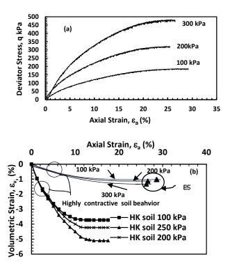
Fig. 3 Results of triaxial tests on plain CDG soil: (a) CID test results, and (b) ( $\varepsilon_a vs. \varepsilon_v$ ) for CID test.
