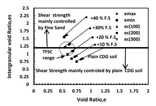
Fig. 8. Limit void ratio for CID tests for: Plain CDG soil , +10 % fine sand , +20% fine sand, +30% fine sand, and +40% fine sand under undrained conditions.
