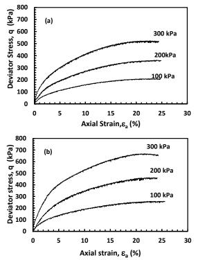
Fig. 4. Deviatoric stress vs. axial strain curves for CID tests: (a) with 10% fine sand, (b) with 40% fine sand.
