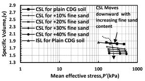
Fig. 9. Steady state lines for CDG soil mixed with different fine sand content for CID test.
