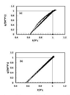
Fig.11. Critical state normalizing for CID tests: (a) with 10 % fine sand, (b with 40 % fine sand.
