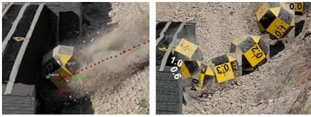
Fig. 8 RC-block trajectory by highspeed images of test No. 7
