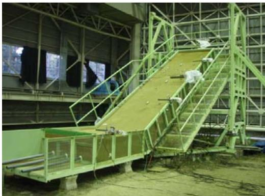
Fig.2 Flume and model slope strain in the slope at 300cm from the toe of the slope, G.W.L. occurred at 5150sec. in the model slope of 30deg.. V.W.C. keeps constant just after the start of the experiment, then and surface displacement at 100cm, 300cm, 500cm from the toe
