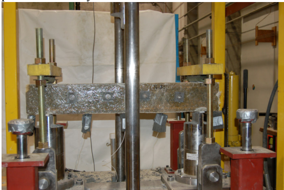
Figure 1. Impact test setup with steel yokes
