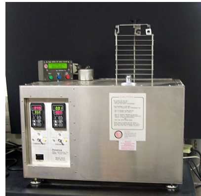
Fig. 3 Pressure Aging Vessel (PAV) for long term aging simulation on asphalt binder
