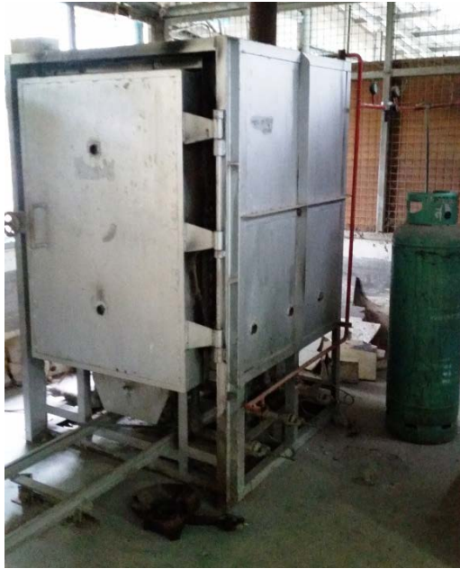
Fig. 4 Kiln fuelled by LPG.
