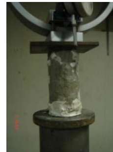
Fig.5 Unconfined compression test on claystone
