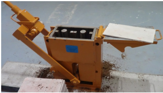
Fig. 2 The manual soil-cement block making press.
